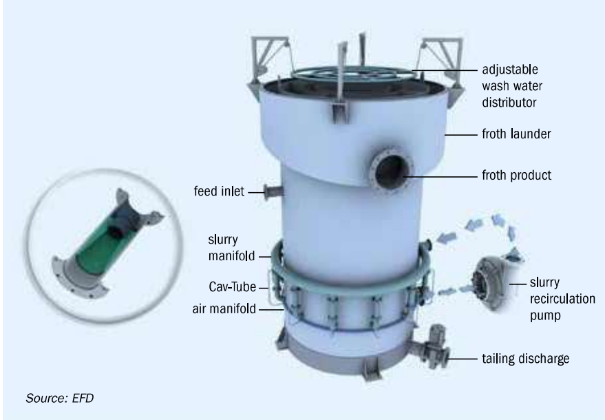
Fig. 1: Typical EFD column flotation cell with cavitation-tube sparging system
